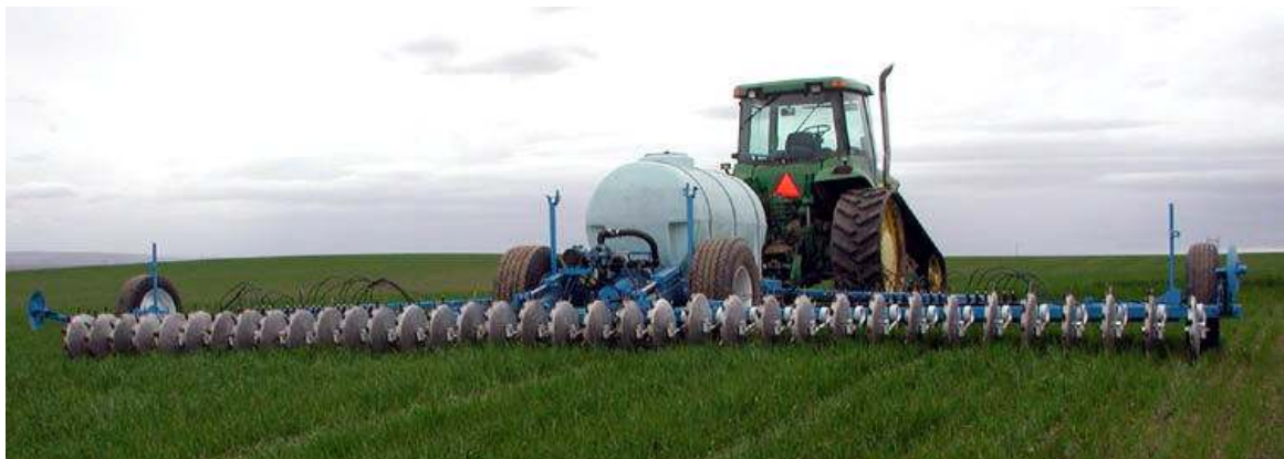
Spikewheel Maschine in Getreide (USA-Oregon)
